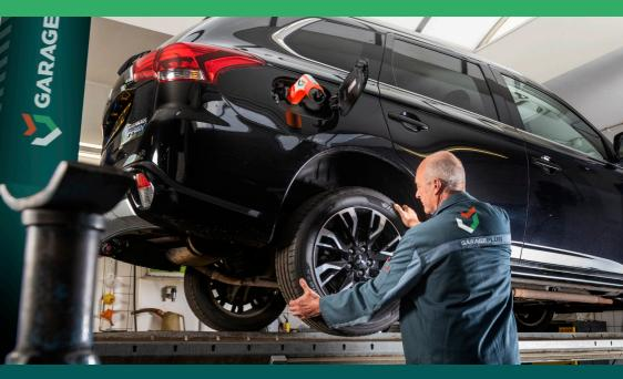
**\_\_\_The Garage Plug** was developed to prevent unpredictable vehicle behaviour during maintenance on an EV. The Garage Plug is compatible with all R100 EV's and provides visual feedback on the connection with the vehicle and whether the plug is working.
